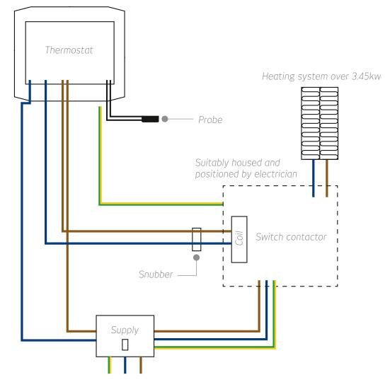
To simplify the operation of the contactor think of it as a switch between the power supply and the heating system.
