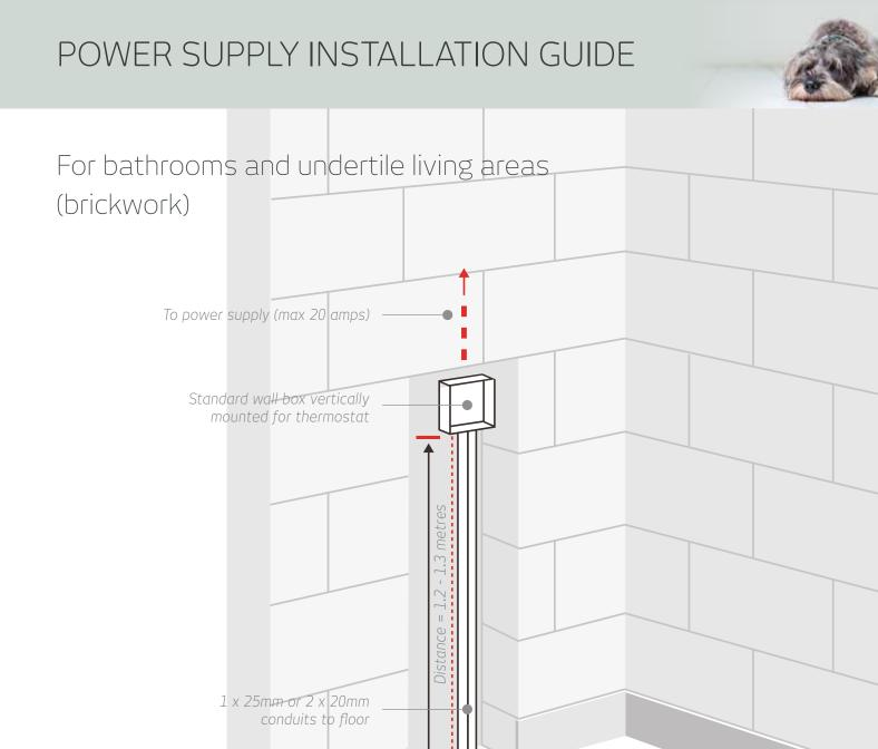
If installing on a double brick wall, draw wire to 20mm hole at floor level is ok.
